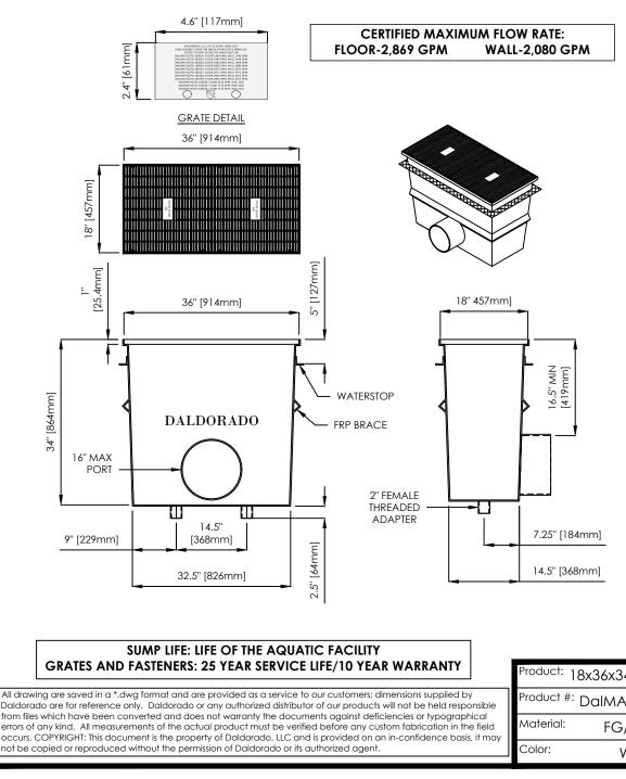
SUMP AND GRATE: UNBLOCKABLE SOFA CERTIFIED TO APSP/ANSI/ICC-16 2017, NSF/ANSI/CAN 50-2020, AND USPC. RPD FIELD CERTIFICATION IS NOT REQUIRED. CORROSION RESISTANT, NON-CONDUCTIVE, NON-MAGNETIC, AND REQUIRES NO BONDING.
